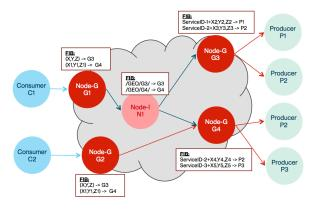
Figure 2b: Geolocation Forwarding over non-GEO intermediate nodes
