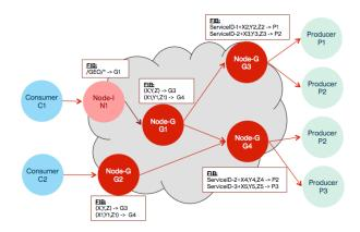
Figure 2a: Geolocation Forwarding with FIB examples for intermediate nodes
