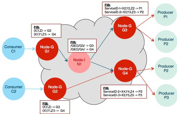
**Figure 2b: Geolocation Forwarding over non-GEO intermediate nodes**
