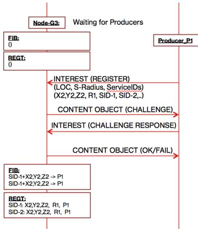
**Figure 1: Geolocation Compass Registration Flows**
