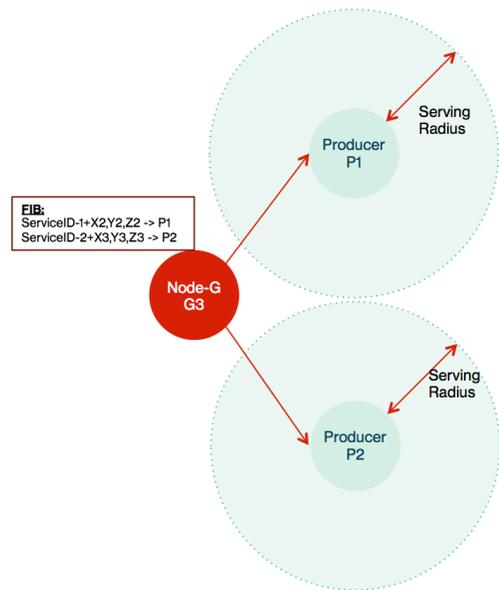
**Figure 4: Geolocation Forwarding with FIB on Edge nodes**
