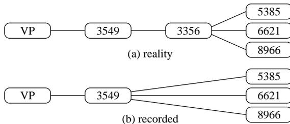
**Figure 4: Transition process merging ASes 3549 and 3356 observed in public BGP data December 2012 to May 2013. To transition the VP into 3356’s network, 3549 used the BGP “local-as” feature so that the neighbor did not have to reconfigure. Customers of 3356 (a) then appeared to be customers of 3549 (b).**
