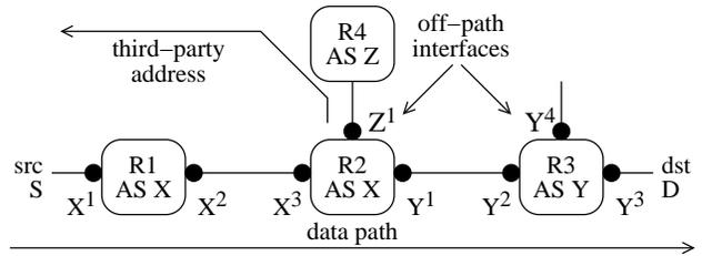
Figure 2: Router-level path between a source S and destination D with off-path interfaces  $Z^1$  and  $Y^4$  labeled.  $Z^1$  is a *third-party address* in this path because it is announced by AS Z which is not in the data path. If R2 replies to a traceroute probe towards D with  $Z^1$ , the derived AS path will be false.
