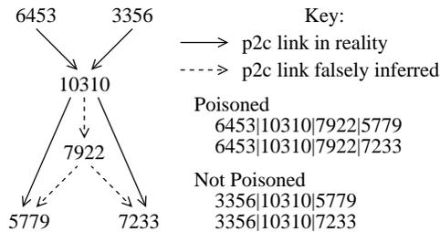
**Figure 3: Path poisoning in AS paths observed in public BGP data during April 2012. AS10310 (Yahoo) inserted AS7922 (Comcast) into routes it announced to AS6453 (Tata) to prevent Comcast selecting a path to Yahoo via Tata. This poisoning causes false link and p2c inferences.**
