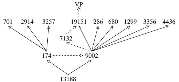
**Figure 8: Triangles inferred using paths in figure 6. The triangles are formed using a path from the misbehaving VP to the same prefix. For the triangle to exist in reality, an AS must receive the same prefix with different paths at different points in their network and then advertise each to different neighbors.**
