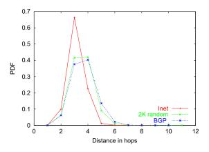
Figure 1: Distance distribution comparing original BGP table data for March 2004, 2K generator, and Inet
