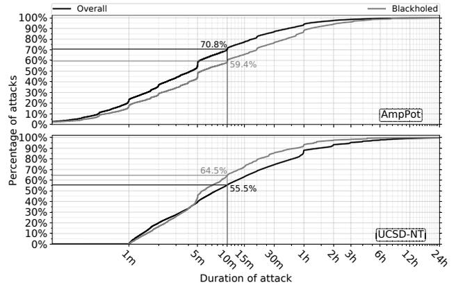
**Figure 5:** the attack duration distributions for all attacks (black curves) and blackholed attacks (gray curves) in the amppot data (upper plot) and the ucspd-nt data (lower plot). we find that for randomly spoofed attacks, the average duration drops, which, given the attack-inference methodology, is indicative that blackholing is effectively stopping (at least part) of victim-destined traffic.
