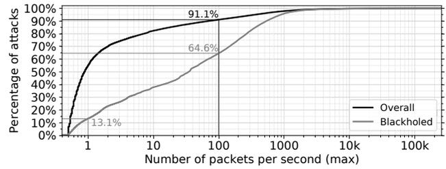
**Figure 3: The intensity distribution for all attacks in the UCSD-NT data set (black curve), as well as for those that are blackholed (gray curve). We show that less intense randomly spoofed attacks are also mitigated – 13.1% see an inferred intensity of at most 3 Mbps (1 packet/s observed).**
