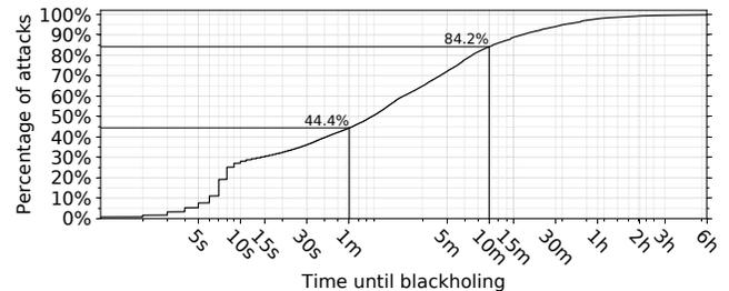
**Figure 1: Time until blackholing is activated. The distribution of the time between the start of attacks and the start of blackholing, for attacks in the UCSD-NT and AmpPot data sets. Almost half of all blackholed attacks (44.4%) see blackholing activated within a minute.**
