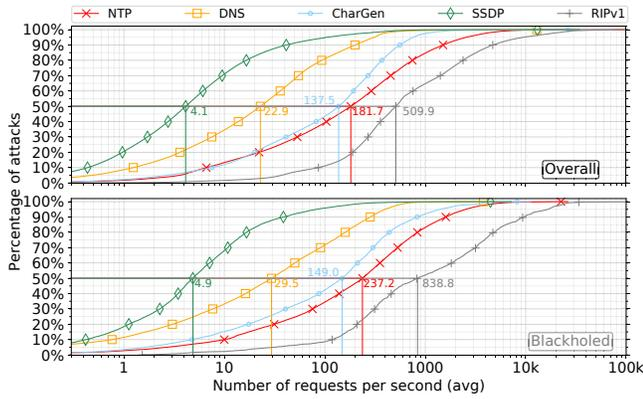
**Figure 4:** For the five most-used reflector protocols, the intensity distribution of all attacks in the AmpPot data set (upper plot), as well as for those that are blackholed (lower plot). We show that less intense reflection attacks are also mitigated. For example, 50% of all blackholed SSDP-based attacks see at most 4.9 requests/s.
