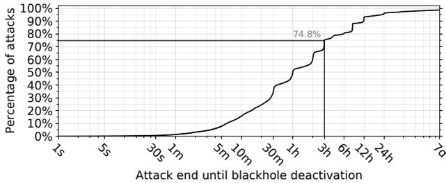
**Figure 2: The distribution of the time between the end of attacks in the AmpPot data set, and the end of correlated blackholing events. In 74.8% of blackholed reflection attacks, the blackholing is withdrawn in three hours or less after the attack stopped. In some cases, however, blackholing is left active for days after.**
