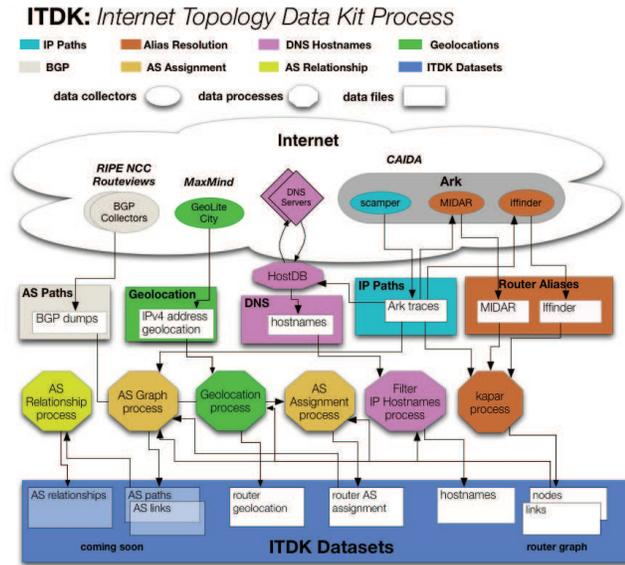
Figure 4: Internet topology data measurement, mining, and analysis process.
