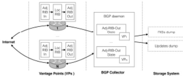
**Figure 1: BGP collection process.** Once a BGP collector establishes a BGP session with a VP, it maintains a state and an image of the VP’s Adj-RIB-out table derived from the updates received through the session. With different periodicity, it dumps (i) a snapshot of all the VP Adj-RIB-out tables (*RIB dump*) and (ii) the update messages received within that period from all the VPs (*Updates dump*).
