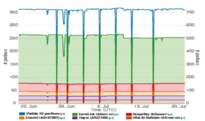
Figure 10: Visible Iraqi prefixes (June, 20- July, 20 2015). Number of prefixes observable in BGP that geo-locate to Iraq (blue line, y2 axis) and number of unique prefixes announced by the 5 top Iraqi providers (stacked lines, y1 axis). An observable series of  $\approx 3$ -hour outages starts on June 27, and ends on July 15. According to the media, the local government ordered complete shutdowns of the Internet service in the country.
