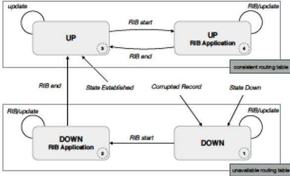
Figure 8: Finite State Machine (FSM) for reconstructing VP routing table. The two macro states (*consistent routing table* and *unavailable routing table*) represent the (un)availability of a consistent routing table. The FSM starts in the *down* state, then it usually moves to *down-RIB-Application*, and, for the vast majority of time, it oscillates between *up* and *up-RIB-Application*.
