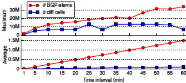
Figure 9: RT diffs vs. BGP elems. Results from running the RT plugin on data from *route-views2* for the month of March 2016: average and maximum number (bottom and top graphs respectively) of BGP elems (red circles) and diff cells published by the RT plugin (blue squares) in each time bin.
