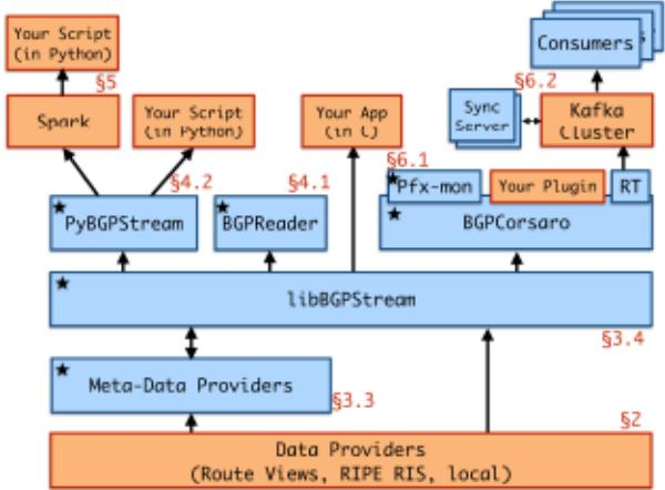
Figure 2: **BGPSStream framework overview.** Blue boxes represent components of the framework; those marked with a star are distributed as open source in the current BGPSStream release [11]. Orange boxes represent external projects or placeholders. Section numbers mark where each component is discussed in this paper.
