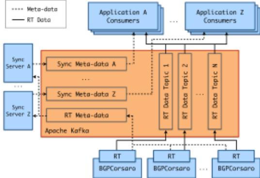
Figure 7: **Distributed framework for live monitoring.** For each collector, we run an instance of BGPCorsaro with the RT plugin which reconstructs the observable LocRIB of all of the collector’s VPs. At the end of each time bin (e.g., 1 minute) each BGPCorsaro publishes diffs to a Kafka cluster. Per-application sync servers then align data from multiple collectors and signal consumers to start processing.
