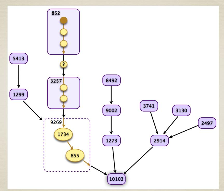
prototype viz showing differences between a traceroute path and BGP AS paths
