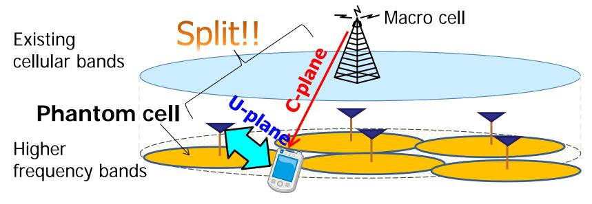
C-plane: Macro cell maintains good connectivity and mobility using lower frequency bands
