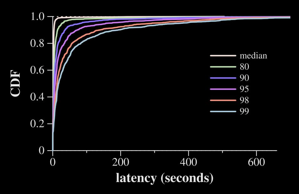
Sampled 2000 of 20k high-rtt IP addresses, sent 1000 pings from our host using scamper. High RTT remains.
