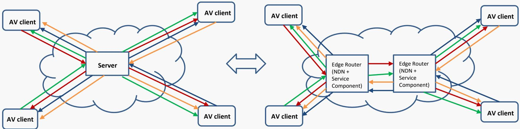
Centralized, IP based: Bandwidth with in the network is  $O(N^2)$  Where N is the number of clients
